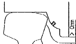
Fig. 67-Template "1W" – bottom part for depth measurement
