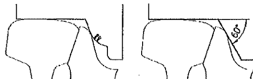
Fig. 66-Template "1W" and grinding template
