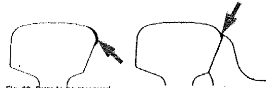
Fig. 69- Burrs to be removed
