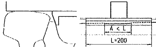
Fig. 68-Templates "2T" and "2L" – Application for switch breakouts
